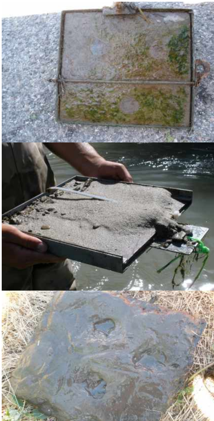
Figure 24. Representative photographs of periphytic algal growth and types of sediment deposition that occur in the Jordan River. Top: Tile retrieved from the river at 5400 South. Middle: Tile retrieved from the river immediately downstream from the 2100 S diversion. Bottom: Tile retrieved from the river in the Legacy Nature Preserve. Note triplicate samples have been collected in the top and bottom photos.
